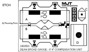
Each etch carries a pair of side frames (A and B) which feature trunions (x) to mount the ends of the torsion wire and tabs (y) which provide two point support for one end of the vehicle. At the other end of the vehicle, the tabs are left 'flat'. Each etch also has a centre bolster (C) and mounting plate (D).
